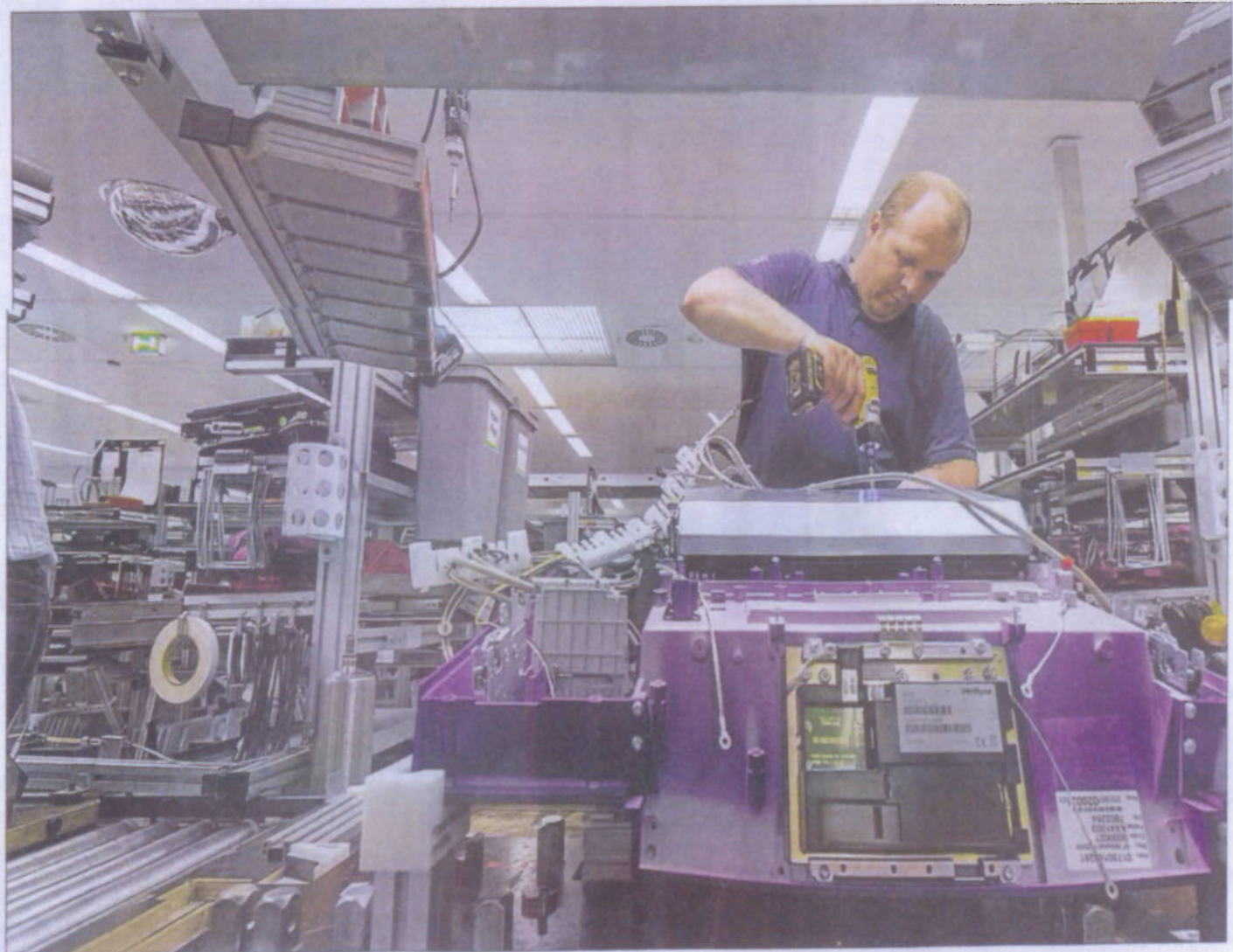
An employee works on the underside of a key pad unit of an automated teller machine on the production line at Wincor Nixdorf in Paderborn, Germany. Picture: BLOOMBERG
